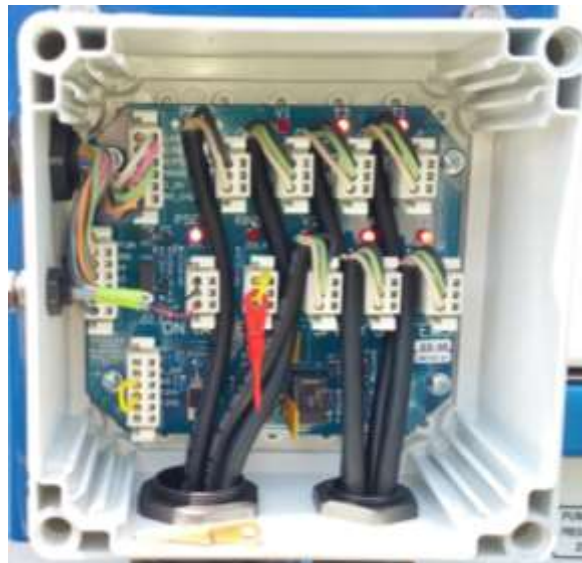
Illustration of Small Junction Box with all Tube lights on
