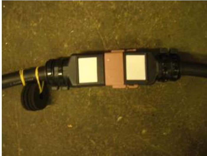
Figure 5: Cord Controller Cord 1 to Junction Box Cord 1 White tape on the same side.
