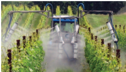
The on-target sprayer is best suited to vineyards with narrow rows.
