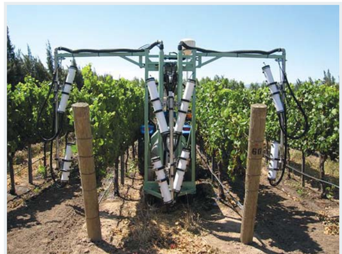
The narrow 32-inch wide sprayer can be configured for two-row application.
