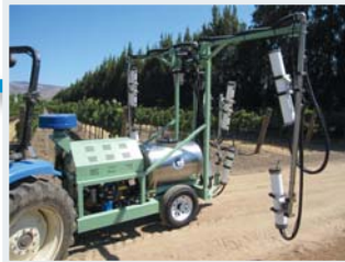
Shown is a sideview of the electrostatic rig and its efficient, lightweight, 70-gallon capacity.
