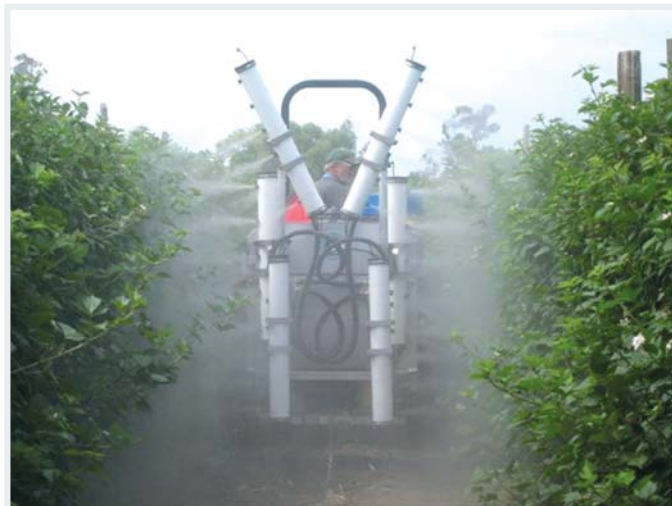
A single-row unit demonstrates targeted low pressure, low volume spray.
