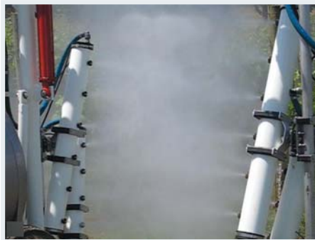
The electrostatically-charged mist will ground to the vines.
