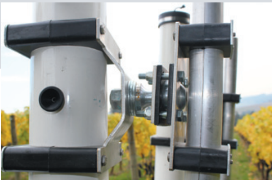
Spray manifolds mounted on ball swivel-clamps afford maximum adjustment.
